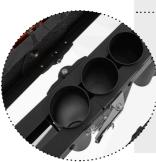
Vancore resonators are individually hand tuned and Vancore resonators are individually hand tuned and assembled using an exclusive mounting system. This system eliminates every kind of rattle. Unlike other resonators, welded or riveted, our system employs minimal contact technology, this eliminates potential problems.
